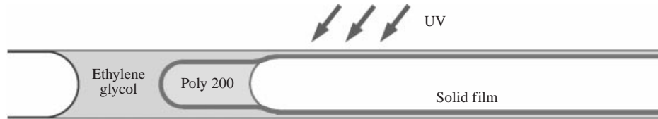
FIGURE 28. UV-cure on light sensitive film and index.
